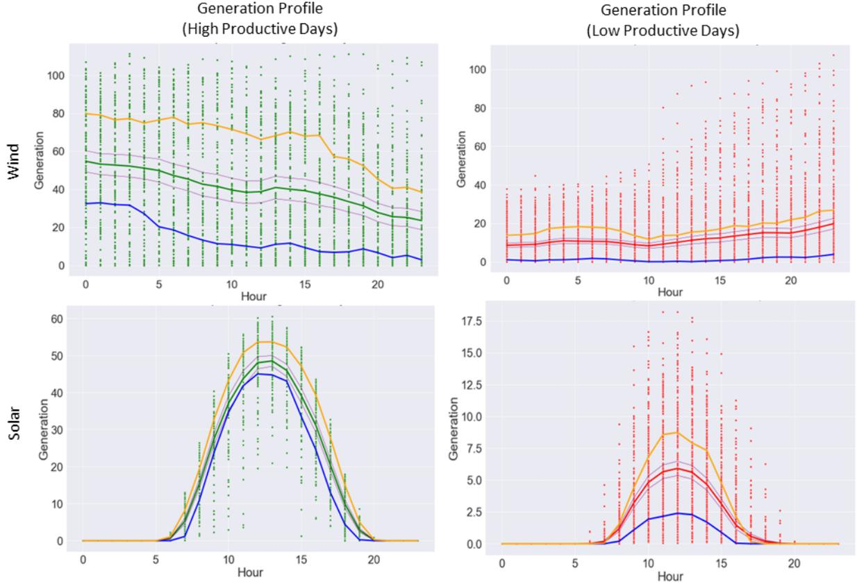
Figure 4: Sample generation profile of high productive (left) and low productive (right) 24 hour periods of wind (top) and solar (bottom) assets generation. The plot shows the mean, 95% confidence on the mean and 5th and 95th percentile of the type of day.
