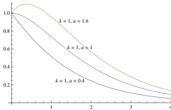
**Figure 1:** the critical damping model
